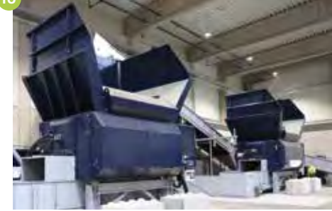
Eggersmann FUEL RDF Production for cement industry Cilacap (IDN) 40,000 t/a household waste Year of construction 2018
