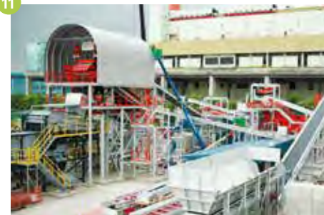
Mechanical slag treatment plant Singapore (SG) 600,000 t/a slag from household waste incineration Year of construction 2015
